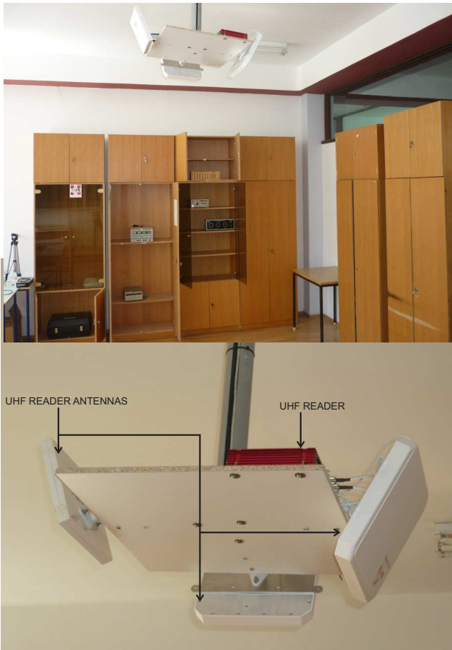
Fig. 4. Measurement and testing set-up
