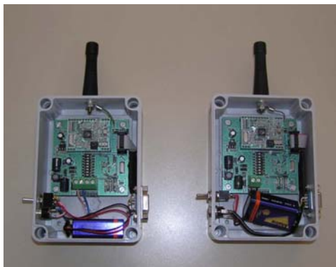
Fig. 3. Implementation of I -codes based on Atmel AT86RF211 transceiver.
