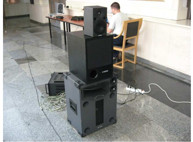
Fig.2. From top to ground: the near-field monitor, the subwoofer and the sound reinforcement loudspeaker.
