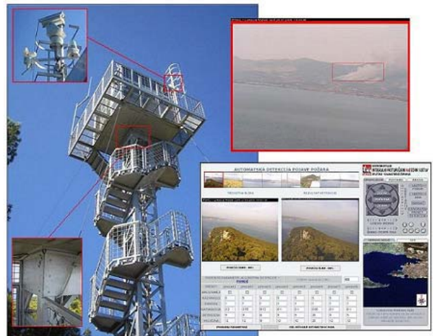
Fig. 3. Monitoring unit and user interface of experimental intelligent forest fire monitoring system iForestFire.
