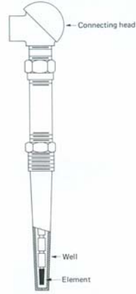
Figure 16.4 Installation assembly for an industrial-type resistance thermometer
