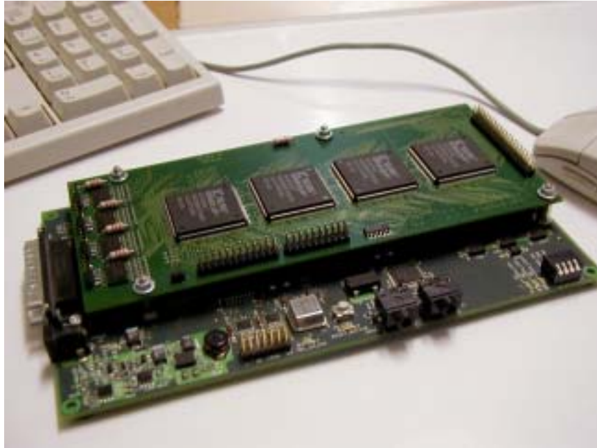
Fig.3. AE module under development.
