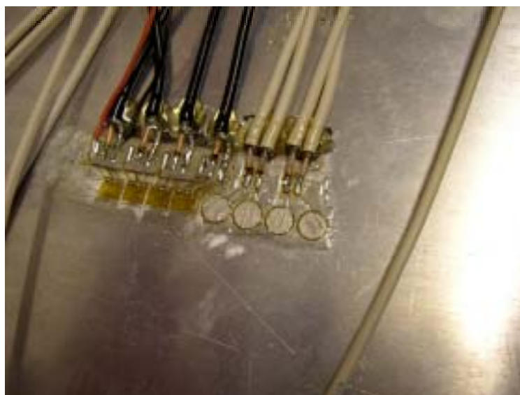
Fig.6. Two four-element phased sensor arrays.
